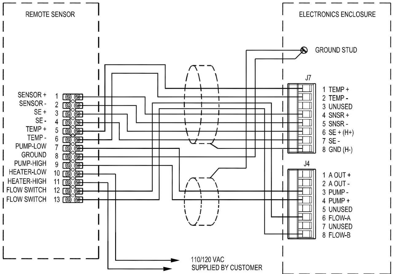
Figure 25: Remote Sensor/Pump Wiring Diagram
