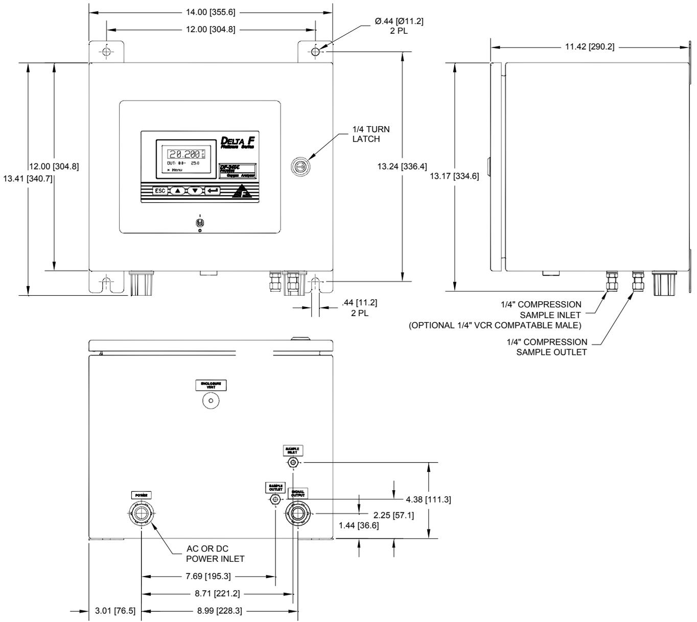
Figure 1: *DF-340E* Oxygen Analyzer
