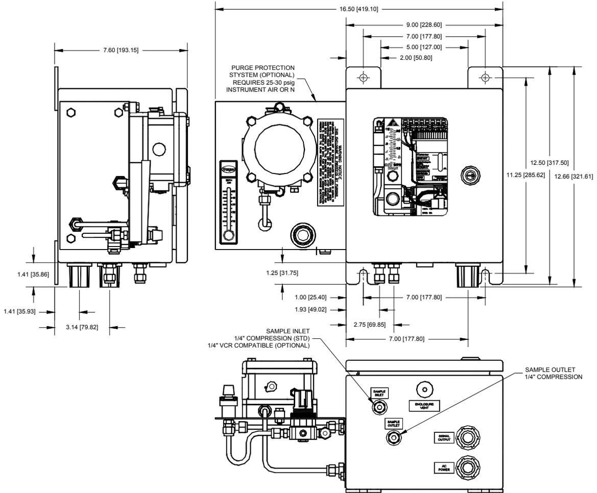
Figure 26: Z-Purge Protection on R4 Sensor Enclosure
