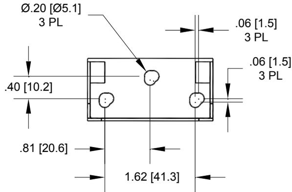
Figure 8: Filter/Regulator Mounting Bracket
