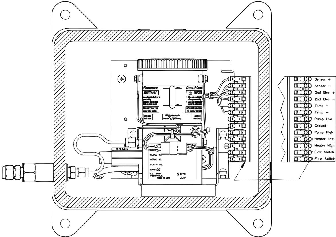
Figure 21: Remote Sensor Mounted in NEMA 7 Enclosure
