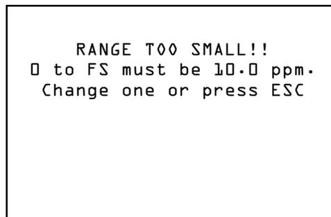
Figure 37: Recorder Output Setup Error
