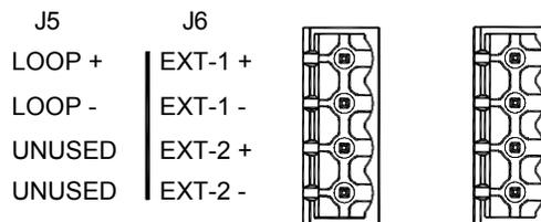
Figure 17: External Control Connector – J6
