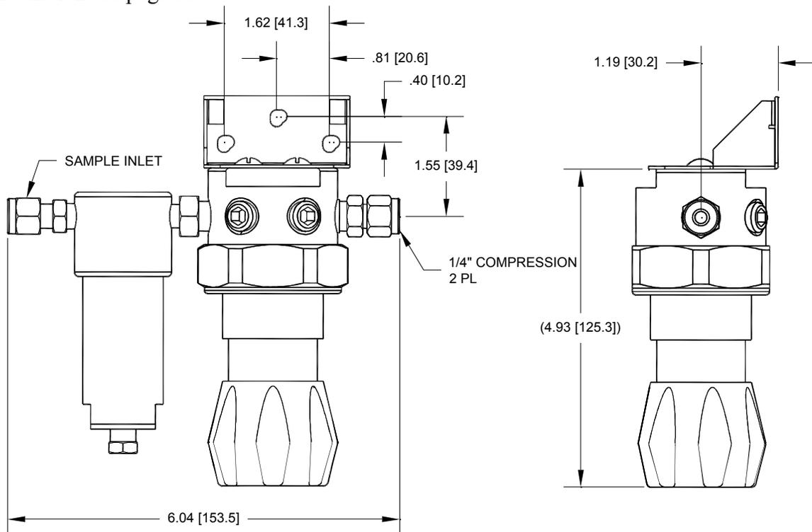
Figure 10: Filter/Regulator Combination and Mount
