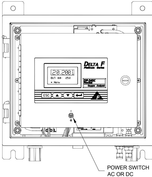
Figure 4: Power Control Switch
