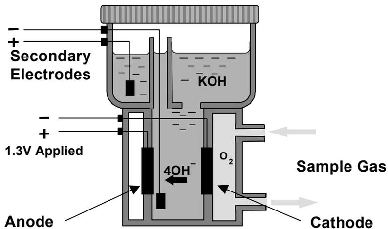
Figure 62: Schematic of Delta F Oxygen Sensor
