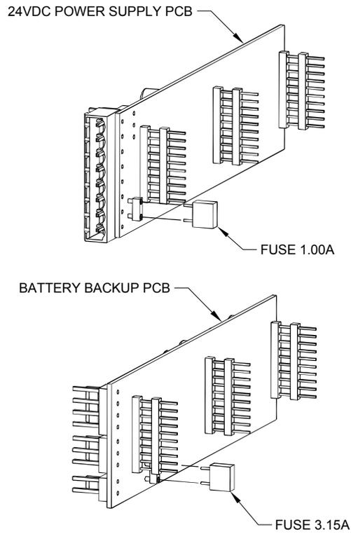
**Figure 60: Fuse Locations for DC Power Supply and Battery Backup**
