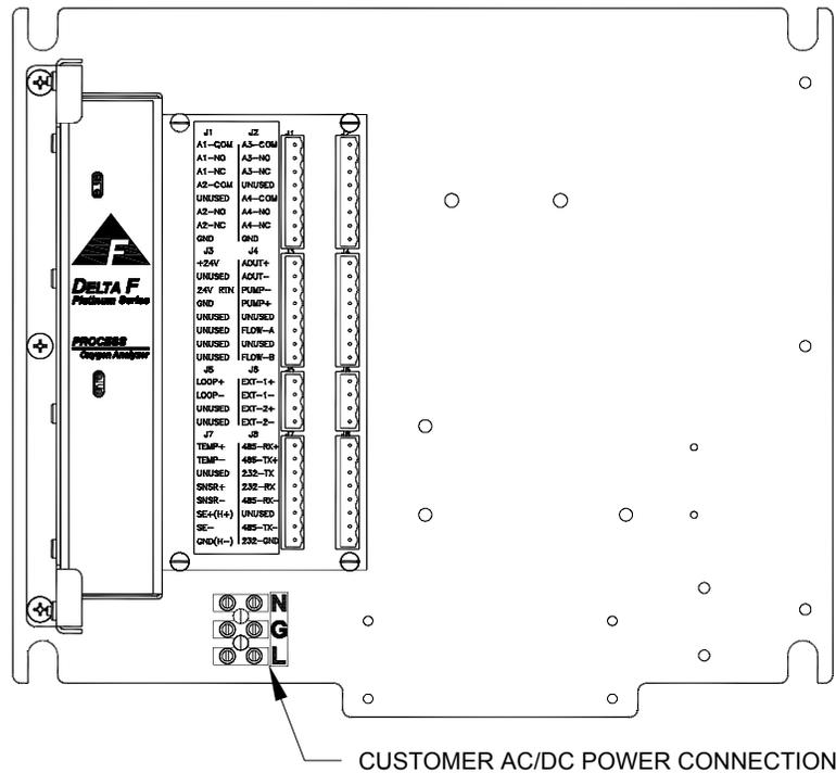
Figure 3: AC/DC Power Input Connections
