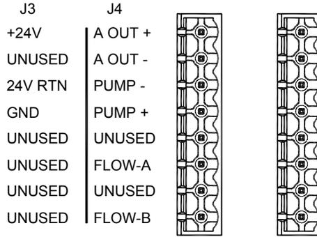
Figure 18: Pump Control Connector – J4
