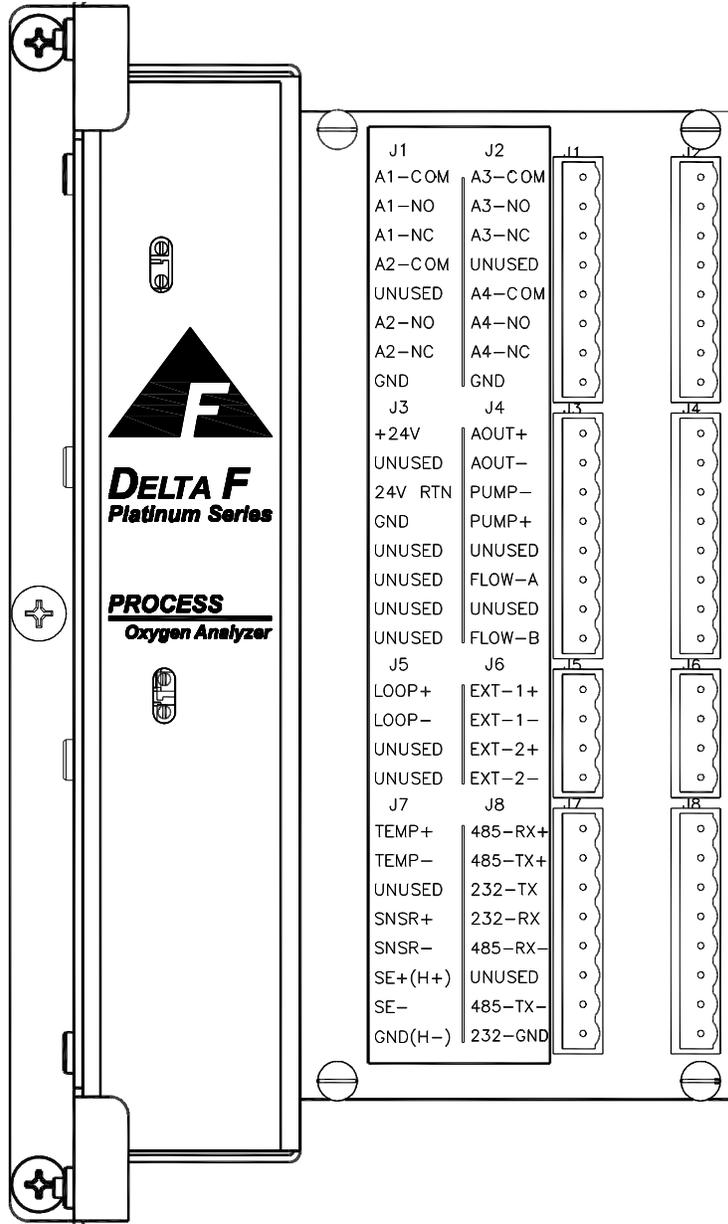
Figure 6: Electrical Connections
