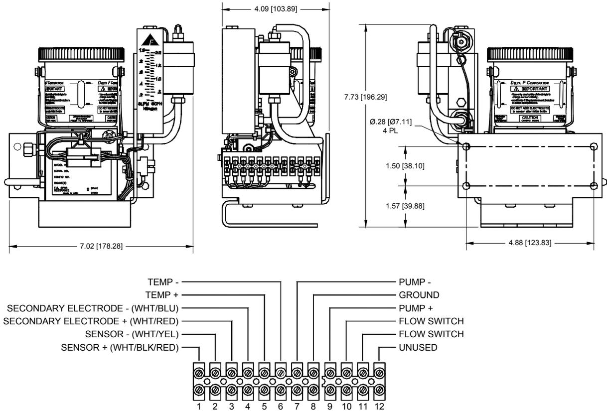
Figure 19: Remote Sensor with Optional Pump
