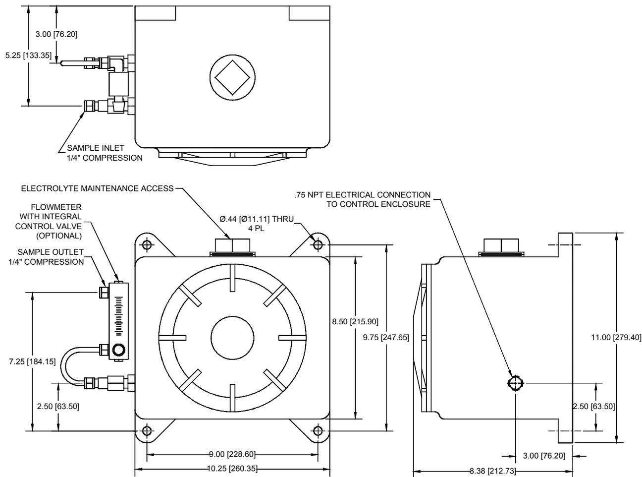
Figure 22: NEMA 7 Enclosure Mounting Dimensions
