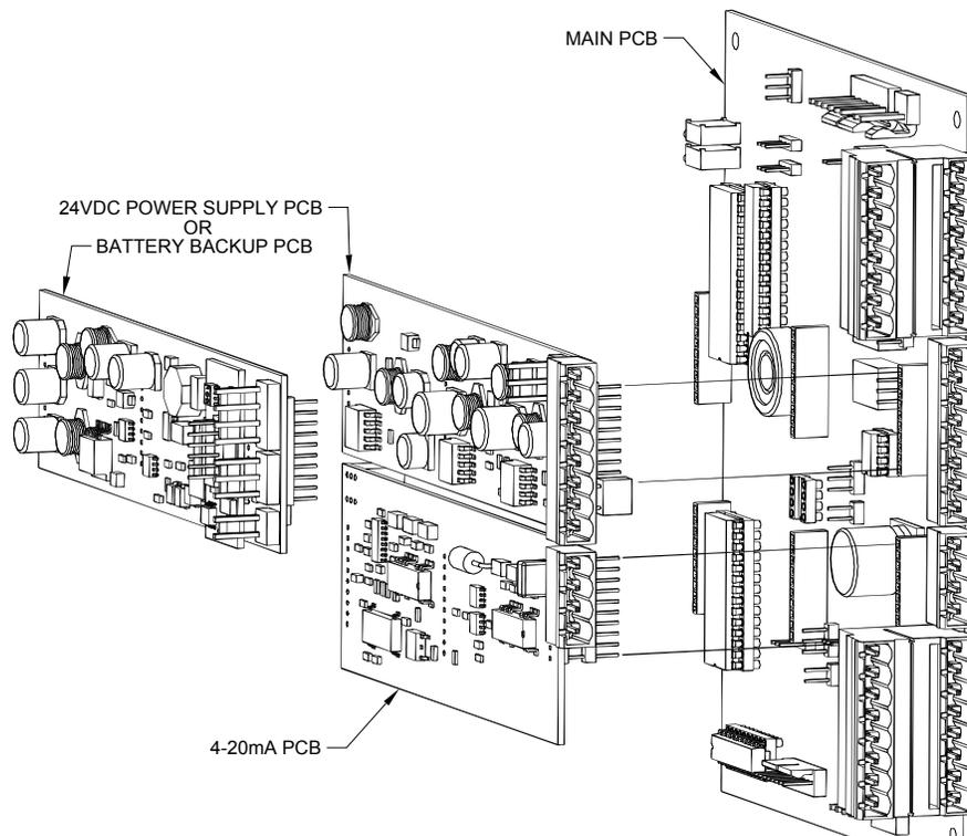
**Figure 61: Printed Circuit Board Assembly**
