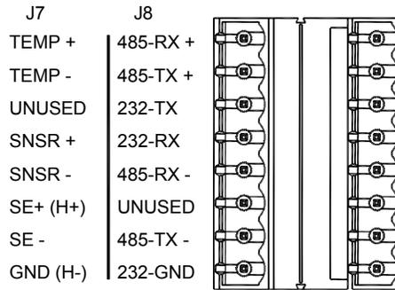
Figure 24: Remote Sensor Connector – J7
