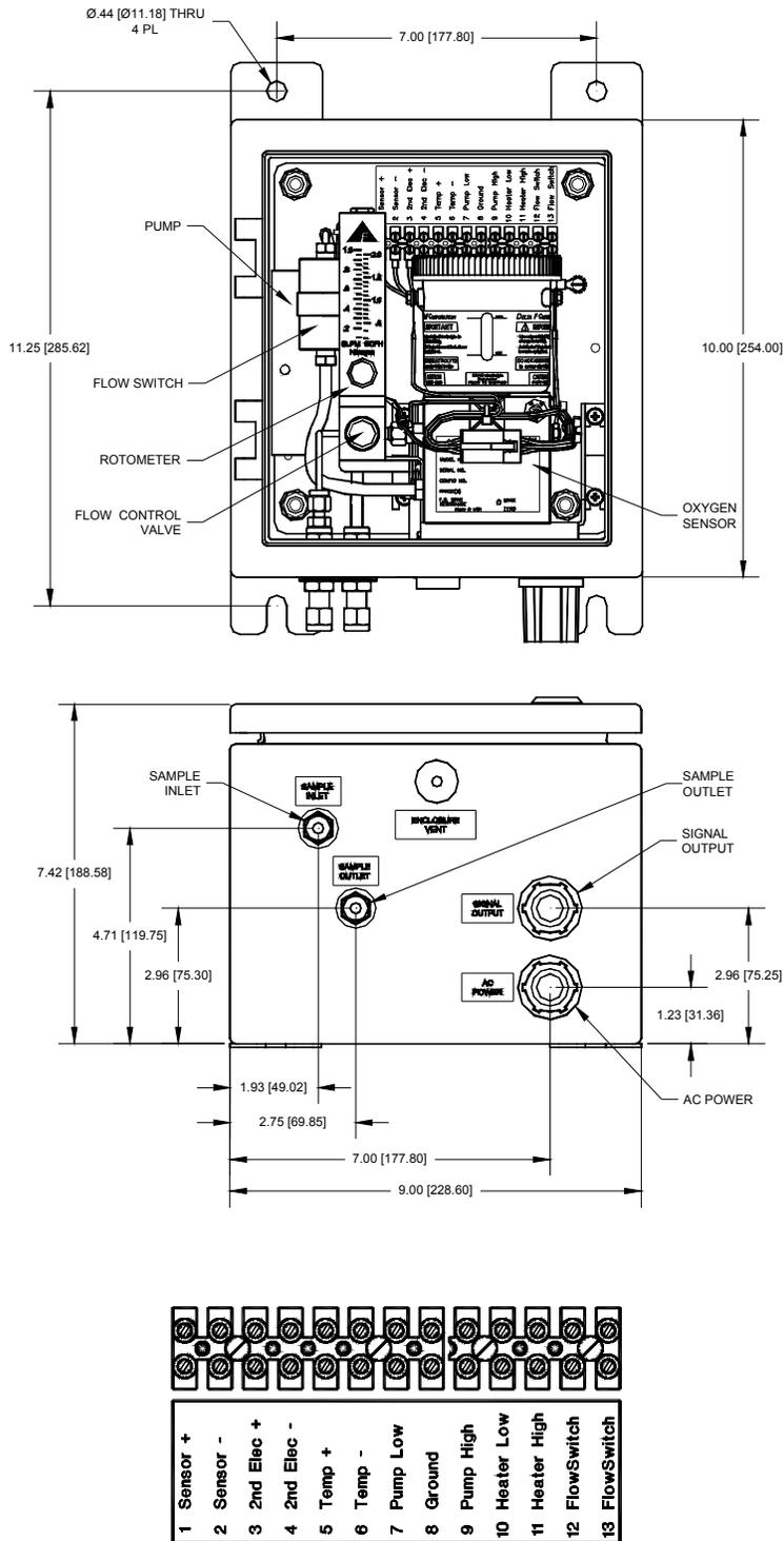
Figure 20: Remote Sensor Mounted in NEMA 4 Enclosure
