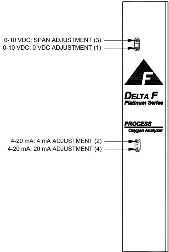
Figure 16: Analog Output/4-20mA Adjustments
